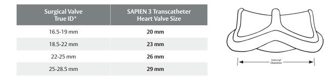
\* Limited bench testing data for explanted calcified surgical valves showed that the measured internal diameter is smaller by ~1-3 mm, compared to 'True ID' for surgical valves.
